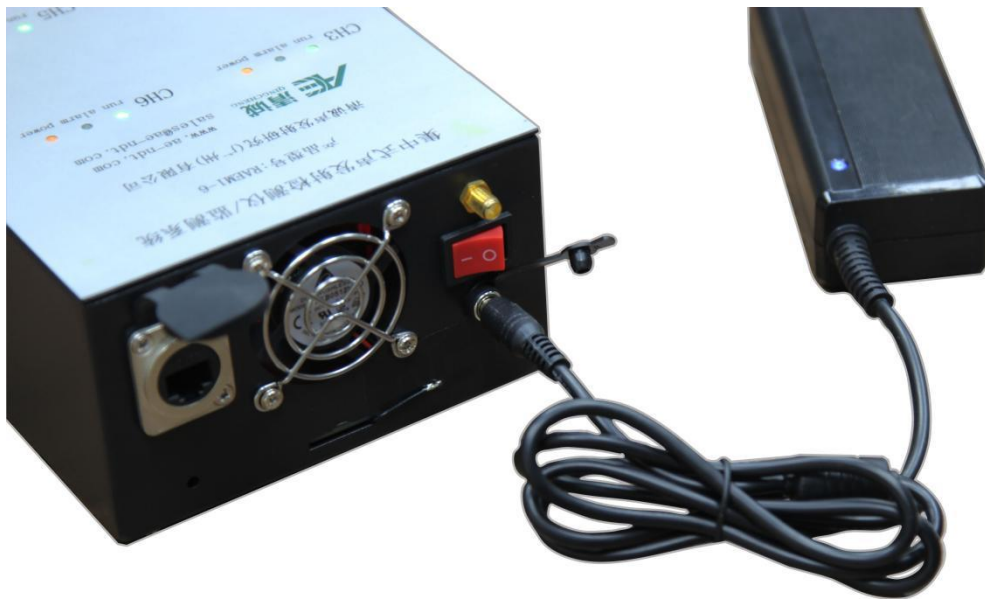
Fig. 2-7 Hardware connection of RAEM1-6 - Rear
