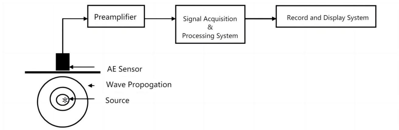
Fig. 1-1 Block diagram of acoustic emission testing principle
