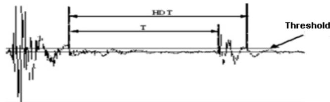
Fig. 3-24 HDT definition diagram
