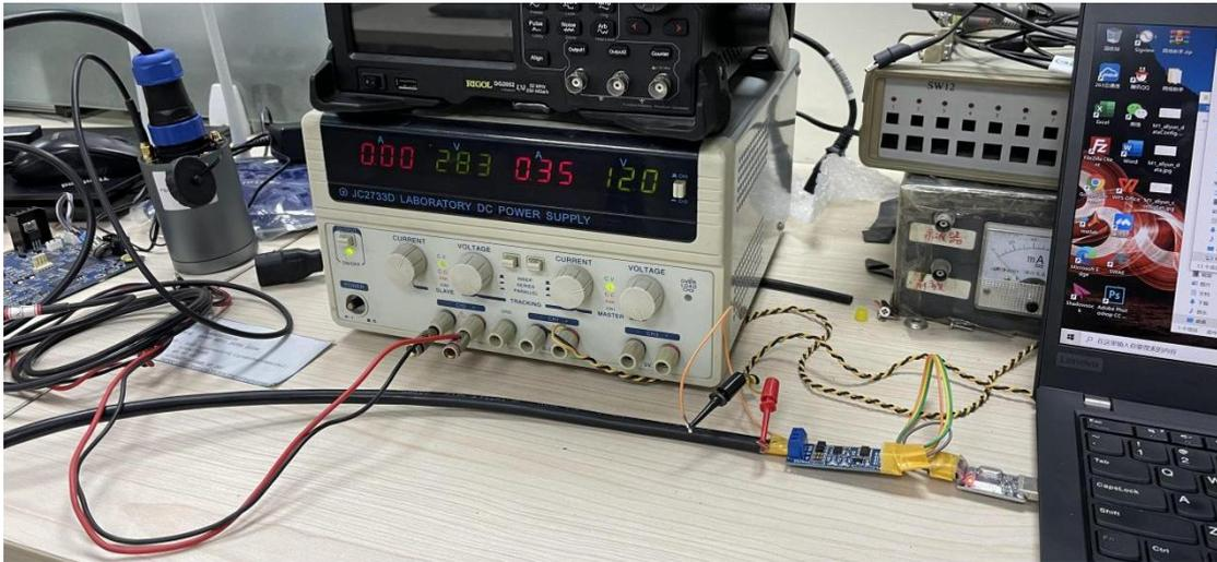
Fig. 7-8 RAEM1 485 hardware test setup
