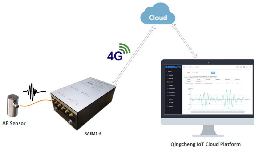
Fig. 3-2 RAEM1-6 Connecting to the cloud over 4G
