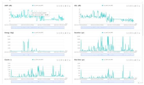
• **AE Feature Parameters:** Arrival time, amplitude, ring count, energy, rise time, duration, RMS, ASL.
