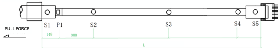
Diagram of the position of cable loading break groove and RAEM position (P1 is the position of broken wire, and S is the position of RAEM1)
