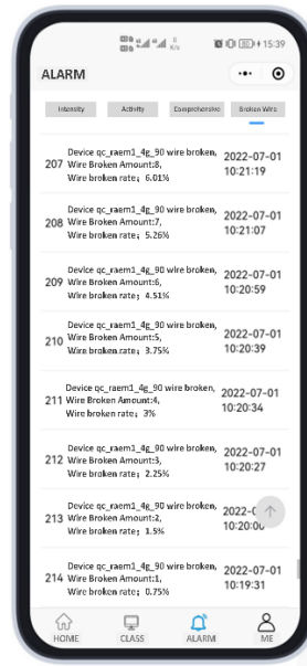
Alarm via APP
